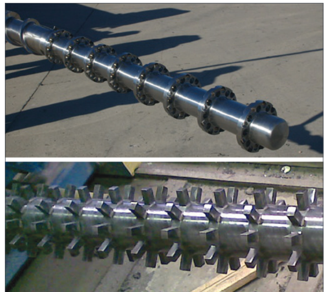
Figure 5: Photos Illustrating some more Commonly Employed Mixing Sections Located at the Melt Delivery End of the Screw
