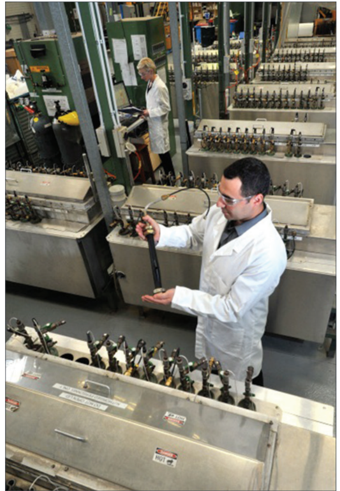
Figure 22: Extensive Hydrostatic Pipe Testing at Qenos Technical Centre
