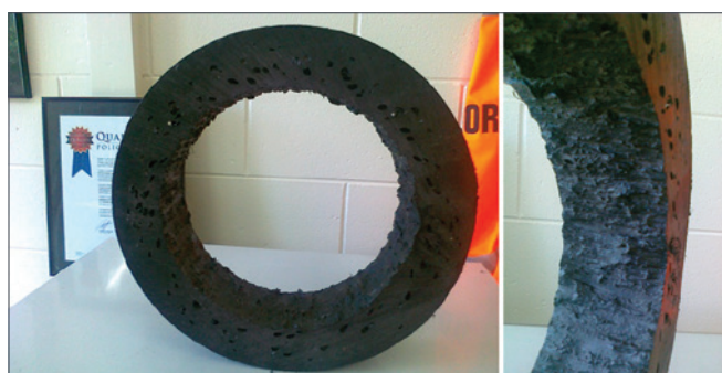
Figure 2: Photograph illustrating a Pipe with Voids and a Rough Pipe Surface due to Excessive Moisture in the Polymer Compound
