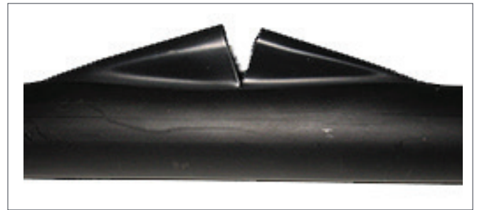
Figure 24: Pipe Failed in Ductile Mode
